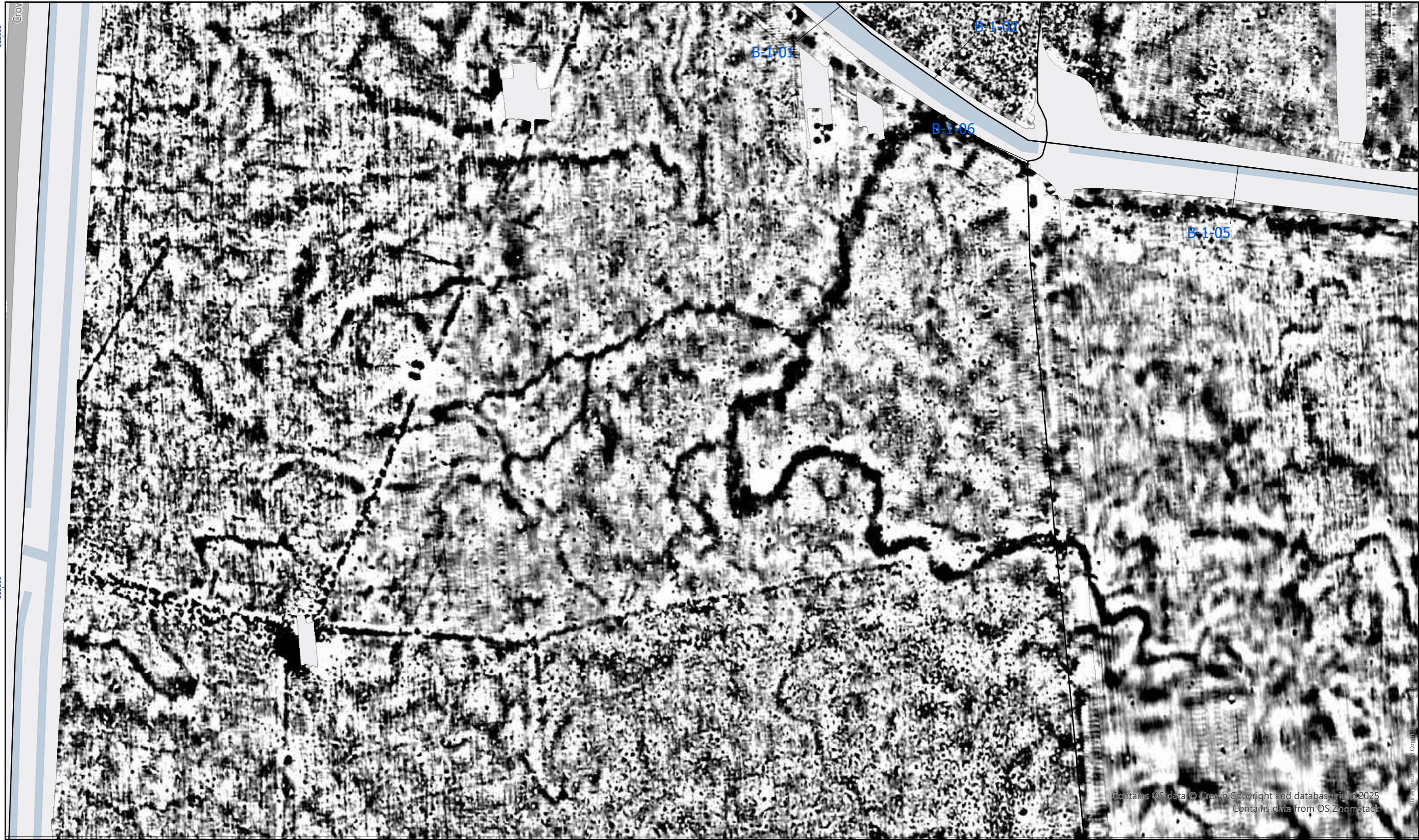
Processed Gradiometer Data – Greyscale Plot - Detailed
